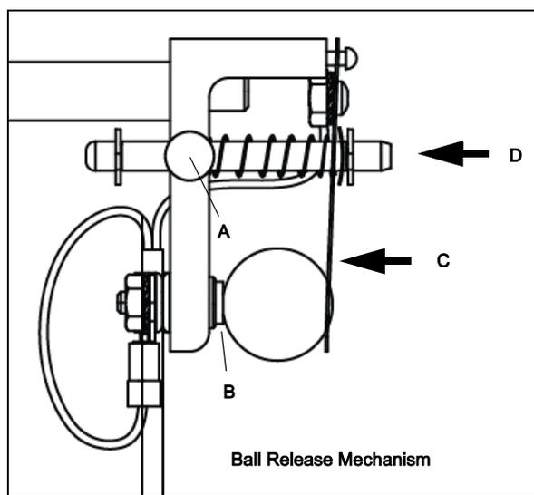
release plate. See B. Press the release plate against the ball to hold it in place. See C.
