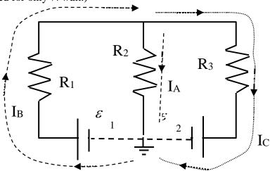
In the figure above the currents have already been drawn in and labeled. Directions for the currents were chosen arbitrarily. The current is the same in any path which does not have a split (junction) in it. Current does not change going through resistors or power supplies -- only at junctions.
