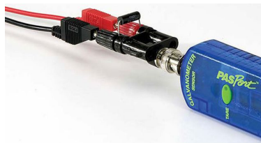
Figure 5: PASPort galvanometer assembly illustration. (Banana plugs are used to connect the galvanometer and solenoid)
