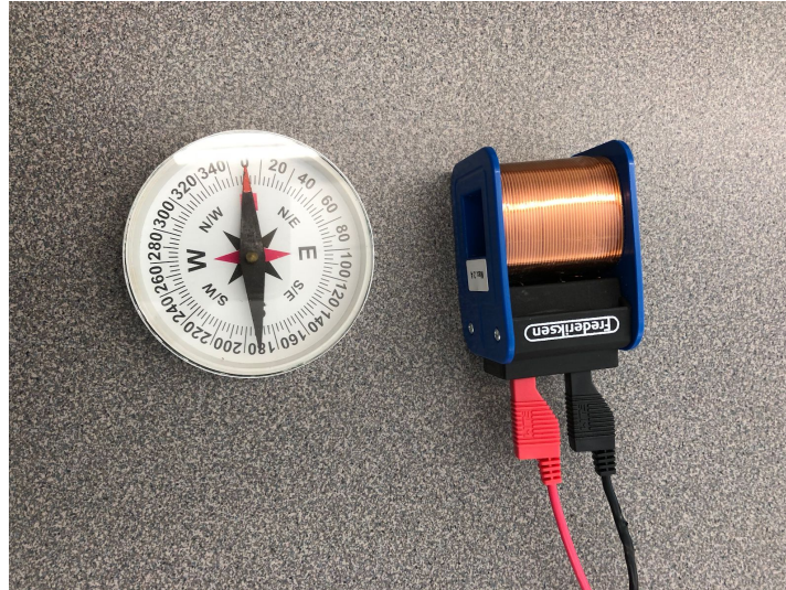
Figure 3. Coil connected to power supply with banana plugs and oriented in the East/West plane (note: no current is running through coil in this image; the compass needle is oriented in the “ambient” magnetic field)
