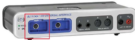
Figure 4: Connect galvanometer to the PasPort 1 input (red).
