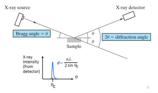
**4.** Continue in this manner, **rotating the Goniometer arm two degrees for every one degree rotation of the crystal**. Record the grazing angle and meter reading at each position.
