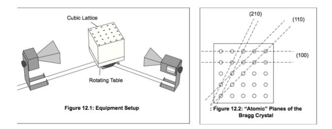
**2.** Notice the three families of planes indicated in **Figure 12.2**. (The designations (100), (110), and (210) are the Miller indices for these sets of planes.) **Measure** the spacing between the metal spheres in your 'crystal' and **calculate** the expected locations (grazing angles) of the n=1 and n=2 peaks for the 100 plane and n=1 peak for the 110 plane. The wavelength of the microwave radiation is 2.85cm.
